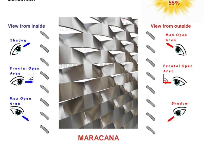
Install a shading means using an item that gives the possibility of shielding all or part of the passage of sunlight while allowing the passage of air. Expanded metal is by nature a material that contains these two features, while having the advantage of being able to add an aesthetic and architectural value to each application.
