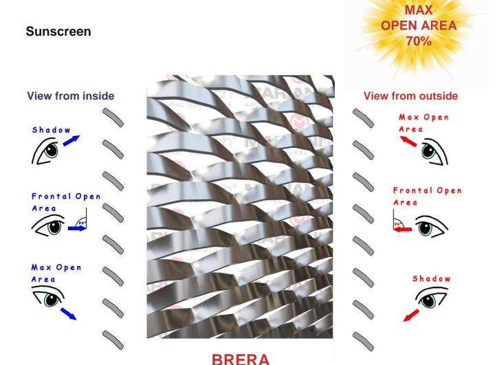
Install a shading means using an item that gives the possibility of shielding all or part of the passage of sunlight while allowing the passage of air. Expanded metal is by nature a material that contains these two features, while having the advantage of being able to add an aesthetic and architectural value to each application.
